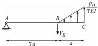
$$\begin{aligned}\sum M_A &= 0 \Rightarrow V_B \times 2a = \frac{1}{2} \left( \frac{Pa}{2EI} \times a \right) \times (2a + \frac{2a}{3}) \\ \Rightarrow V_B &= \frac{Pa}{3EI}\end{aligned}$$
