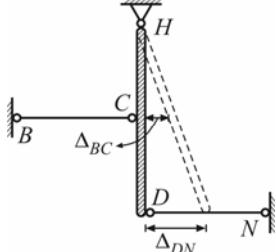
$$\begin{aligned} & \text{رابطه سازگاری: } \Delta_{DN} = 2\Delta_{BC} \\ & \Rightarrow \frac{F_{DN}L}{EA} = 2(\alpha\Delta TL - \frac{F_{BC}L}{EA}) \end{aligned}$$
