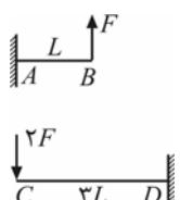
$$\left\{ \begin{array}{l} \Delta_B = \frac{FL^3}{3EI} \\ \Delta_C = \frac{\gamma F(\gamma L)^3}{3EI} = \frac{18FL^3}{EI} \end{array} \right. \Rightarrow \theta_{BC} = \frac{\frac{FL^3}{3EI} + \frac{18FL^3}{EI}}{2L} = \frac{55FL^3}{6EI}$$
