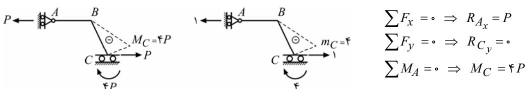
$$\Delta C \times 1 + 0 = \int \frac{M(x) m(x)}{EI} dx = \frac{A_M \bar{m}}{EI} = \frac{\left[ \frac{1}{2} (4P \times 5) \right] \times \left( \frac{2}{3} \times 4 \right)}{EI} = \frac{80P}{3EI}$$
