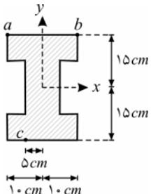
$$\sigma_a = E \varepsilon_a \Rightarrow \frac{T}{A} + \frac{M_x \times 15}{I_x} + \frac{M_y \times 10}{I_y} = 15 \times 10^{-3} E \quad (1)$$
