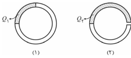
$$\begin{cases} \tau_{max_1} = \frac{VQ_1}{It}, Q_1 = (A\bar{y})_1 = \frac{\pi}{4}Rt \times \frac{2R}{\pi} = R^2t \\ \tau_{max_2} = \frac{VQ_2}{It}, Q_2 = (A\bar{y})_2 = \pi R t \times \frac{2R}{\pi} = 2R^2t \end{cases}$$
