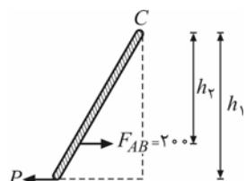
$$\begin{cases} \sum M_C = 0 \Rightarrow Ph_1 = F_{AB}h_2 \Rightarrow P = F_{AB} \frac{h_2}{h_1} \\ \frac{h_2}{h_1} = \frac{150}{200} = \frac{3}{4} \end{cases} \Rightarrow P = 200 \times \frac{3}{4} = 150$$
