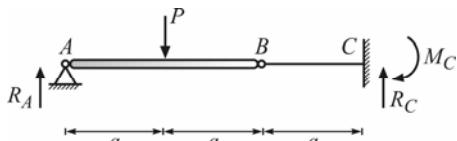
$$\begin{aligned}\sum M_{BL} &= 0 \Rightarrow R_A \times 2a = P \times a \Rightarrow R_A = \frac{P}{2} \\ \sum F_y &= 0 \Rightarrow R_C + R_A = P \Rightarrow R_C = P - \frac{P}{2} = \frac{P}{2} \\ \sum M_{BR} &= 0 \Rightarrow M_C = R_C \times a = \frac{Pa}{2}\end{aligned}$$
