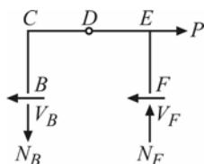
$$\begin{aligned}\sum M_F &= 0 \Rightarrow N_B \times 2L = P \times L \Rightarrow N_B = \frac{P}{2} \\ BCD : \sum M_D &= 0 \Rightarrow N_B \times L = V_B \times L \Rightarrow V_B = N_B = \frac{P}{2}\end{aligned}$$
